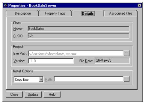
Use the Details tab to provide a description and technical details about the selected <u>component</u>.
