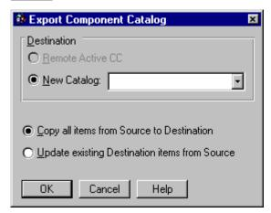
Use the Export Component Catalog dialog box to synchronize the contents of one component catalog with another. This is generally used to create a portable component catalog for use when you work on a stand-alone computer, such as a laptop, and don't have access to remote catalogs on the network.
