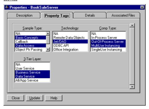
Use the Property Tags tab to select global information relating to all classes in a <u>component</u>, or all members in a class, by setting the properties on the component and class, respectively.
